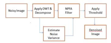
Fig.4: Block Diagram explaining sub band adaptive thresholding with neighbourhood pixel filtering
